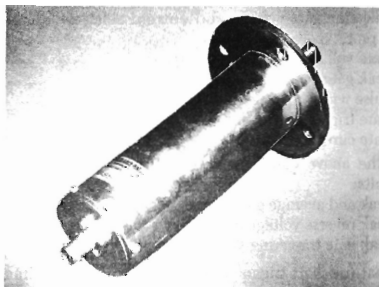
FIGURE 21.4 A COMMERCIAL NON-INDUCTIVE CURRENT SHUNT
